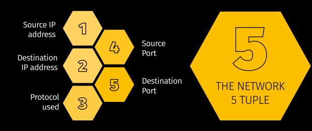
Full-Packet Capture: Consists of the entire packet - including the 5-tuple data as well as the full packet payload, such as the query and response data, industrial commands, function codes, and other artifacts. Even files in the packet payload may be extracted for analysis during incident response cases, such as malware samples. Full-packet capture does consume significantly more storage space than just capturing 5-tuple data.
